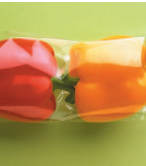
ABOVE: Fruit bowl and BELOW: Biophan® film, both made from polyactic acid, derived from corn starch/sugar
