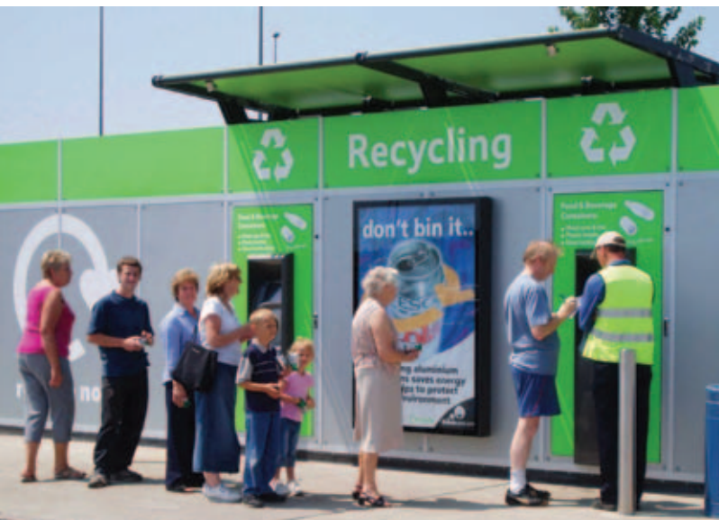
Tesco's TOMRA recycling machine uses infra-red real-time technology to sort up to 80 items per minute (see box, p50).
